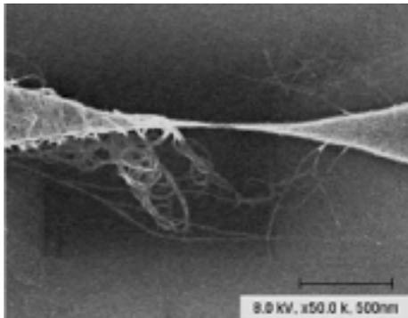
*Particle sensor formed with a broken nanotube. Courtesy of Mechanical Engineering department, Northwestern University.*
