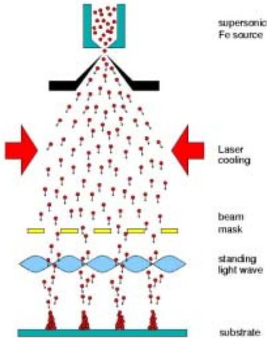
*Atom lithography scheme. Courtesy Roel Bosch, Atomic Collisions and Quantum Electronics Group, Eindhoven University of Technology*
