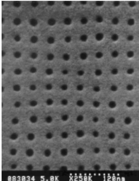
*SEM micrograph of a top view of 60nm deep holes imprinted into PMMA which have a 10 nm minimum diameter. Courtesy Nanostructure Laboratory, Department of Electrical Engineering, University of Minnesota.*
